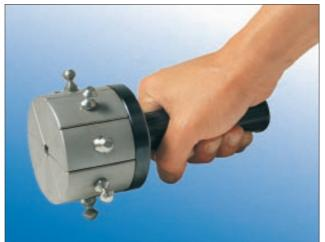
The quick change tool, available as an option for the swagers, allows the whole die set to be changed in one easy operation. The pins on the tool engage the holes in the dies. As the swaging head closes/opens the dies are secured to/released from the master dies. The dies are held together by a magnet in the tool until the set is placed back in the rack. This way the dies are kept in complete sets at all times and are always used in the same order.
